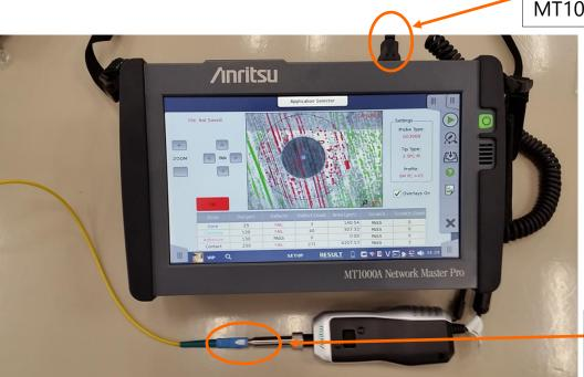
**1.** The VIP USB terminal is connected to the MT1000A/MT1040A series instrument's USB port.
