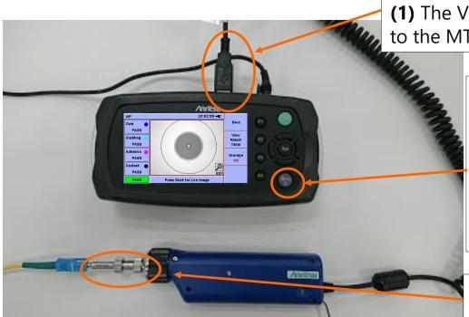
(1) The VIP USB terminal is connected to the MT9090A's USB port.
