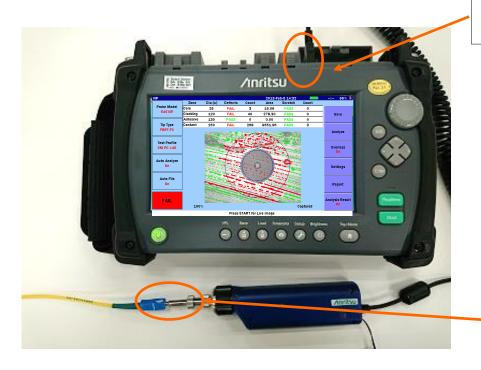
**1.** The VIP USB terminal is connected to the MT9083x2 series instrument's USB port.
